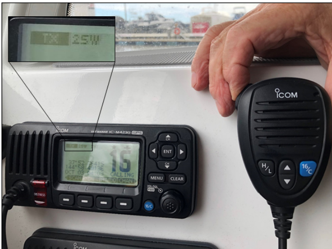
Figure 4: A VHF Marine Radio transmitting at 25W
